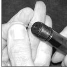
STEP 17 Reinstall the LAMP (8) in the receptacles of the UPPER INSULATOR (10). Adjust the LAMP (8) so it is as vertical and straight as possible. Using a clean soft cloth, gently wipe the moisture and oil from the glass on the LAMP (8).
