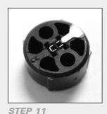
The LOWER INSULATOR (15) should look like this. Note that the SIDE CONTACT (13) comes to the rim of the insulator.
