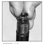
STEP 16 While firmly holding the TOOL and BARREL (12), line up the pins of the UPPER INSULATOR (10) with the holes of the LOWER INSULATOR (15).
