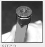
To separate the SWITCH ASSEMBLY (21) prior to installation, place the SWITCH ASSEMBLY (21) on the LONG PIN TOOL.
