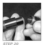
Reinstall TAIL CAP ASSEMBLY (16) always make sure tail cap is tight for a good positive electrical contact. Call Warranty if problems persist. Tel: (800) 283-5562 or (909) 947-1006
