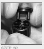
Push down on the lower half of the SWITCH ASSEMBLY (21), this will cause the UPPER INSULATOR (10) to pop up.
