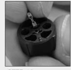
STEP 13 If this happens, carefully place the SIDE CONTACT (13) into the hole, making sure the fan portion of the SIDE CONTACT (13) extends towards the rim of the LOWER INSULATOR (15). The two lamp pin holes must be visible.
