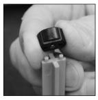
STEP 14 Place the LOWER INSULATOR (15) with the SIDE CONTACT (13) facing up, on the short pin end of the tool make sure the pins of the tool are in the holes of the LOWER INSULATOR (15).
