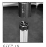
Insert the TOOL with the LOWER INSULATOR (15) into the bottom of the BARREL (12). Push the TOOL into the BARREL (12) until it stops at the top of the BARREL (12).
