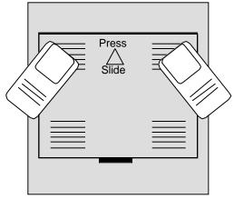
**Battery Installation** Uses four (4) AA batteries. Hold nFOCUS upside down with white adjustment knobs down. Insert arrowed end of access plate under lip of opening with arrow pointing down. Press down on access plate and slide upwards until securely attached.
